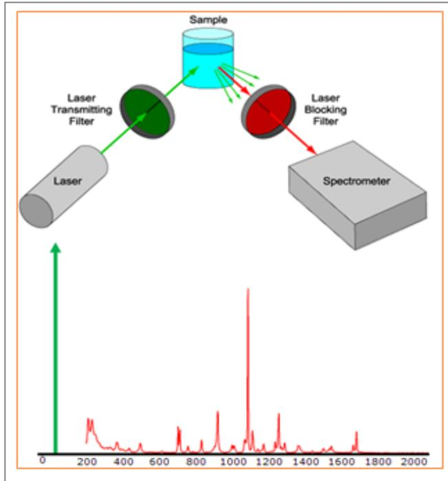
Figure 3: Raman Spectrum – the green line is the laser and the red line is the Raman spectrum (fingerprint) of the sample.
